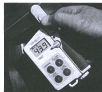
Figure 5. Example of chlorophyll meter on leaf.
