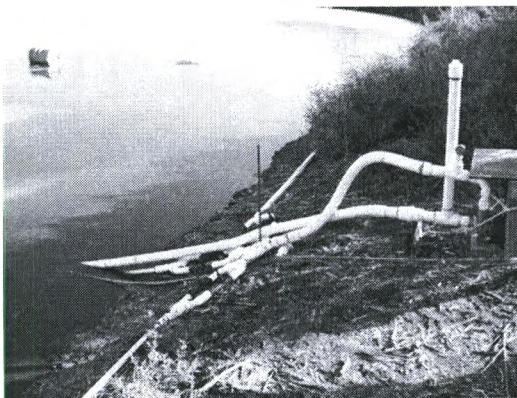
Figure 2. The aerator module in the field test
