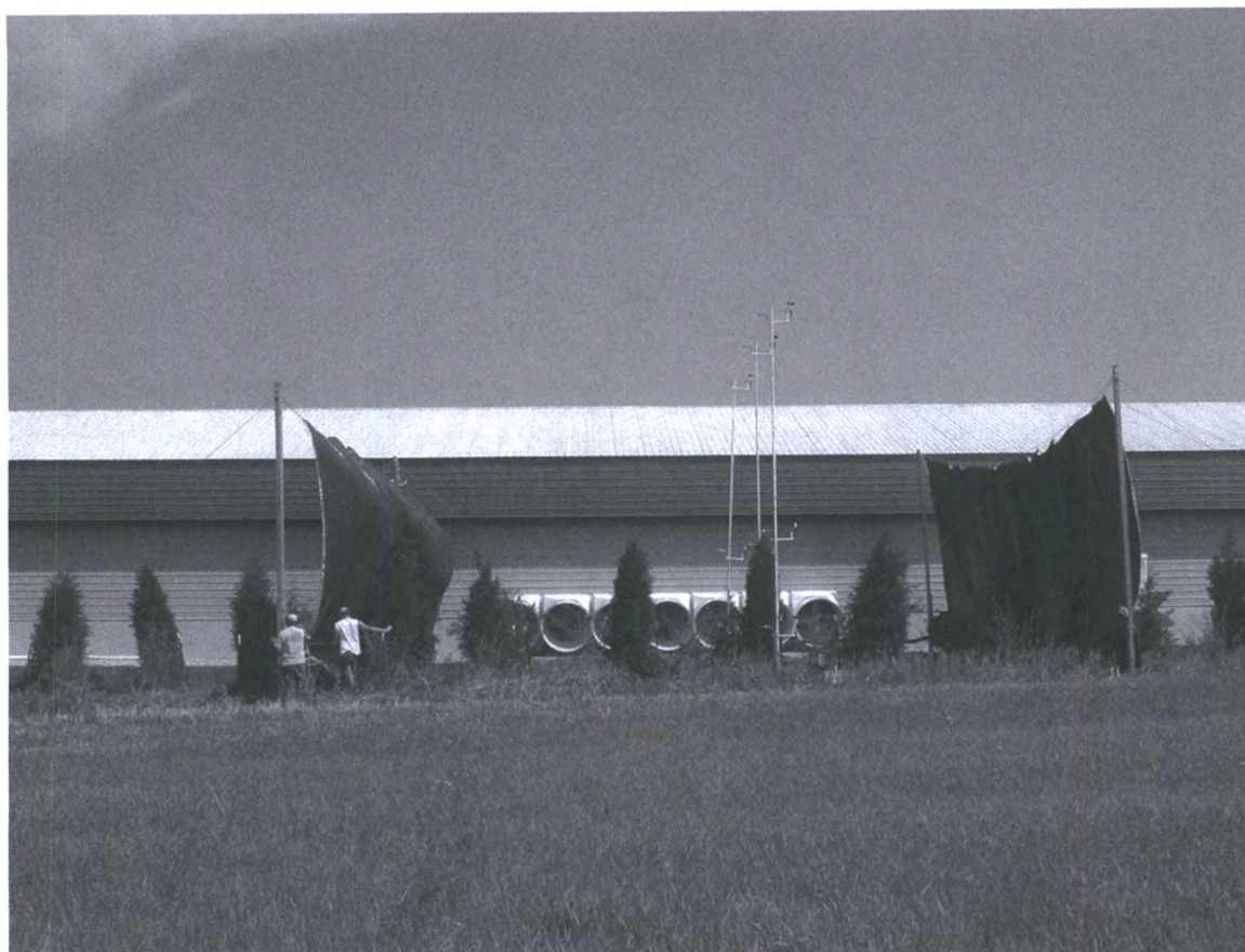
Figure 3. PMT set-up with sampling diversion curtains extended
