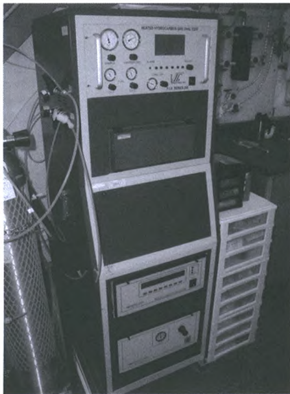
Figure 3. Gaseous emission monitoring instruments in MAEMU.
