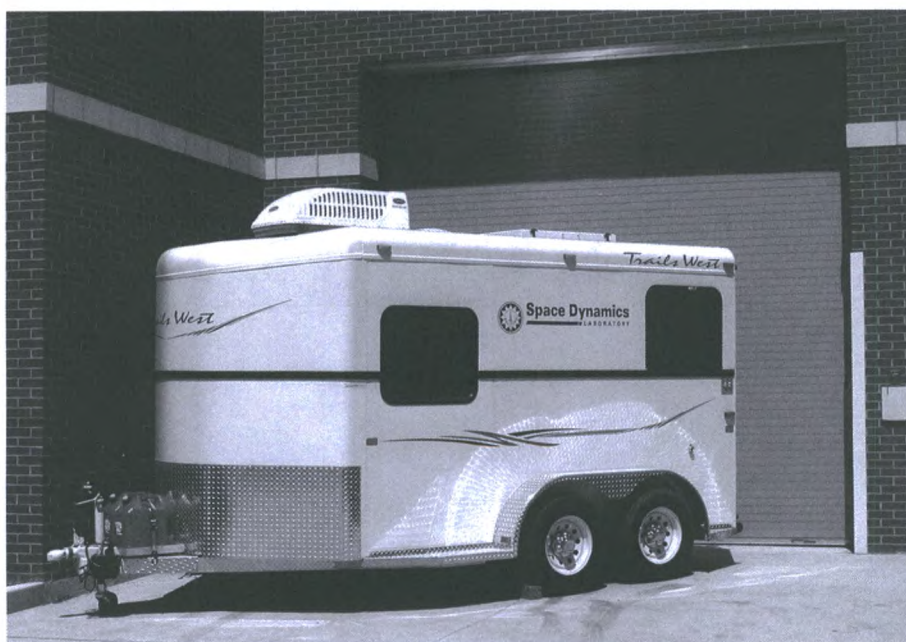
Figure 3. Field deployment trailer for AGLITE lidar
