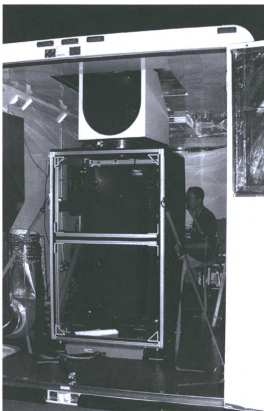
Figure 2. AGLITE lidar mounted vertically, viewed through open back door of trailer
