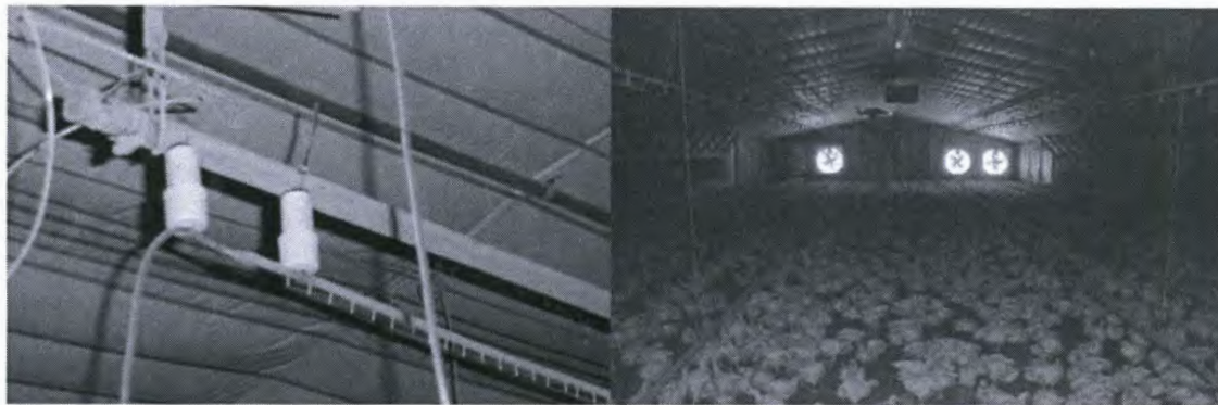
FIGURE 1. Electrostatic space charge system (ESCS) in-line ionization units hanging from the ceiling of the Treatment House (TH). Four units, two in the brood end and two in the growout end were hung on either side from the center of the house.
