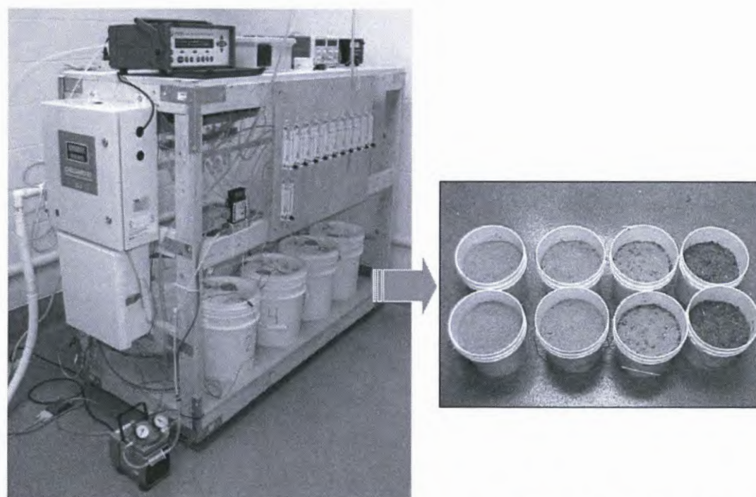
Figure 2. Photographical views of the lab-scale setup for evaluating efficacy of air emission mitigation strategies. Pictured (right) is topical application of zeolite on laying hen manure at various dosages.
